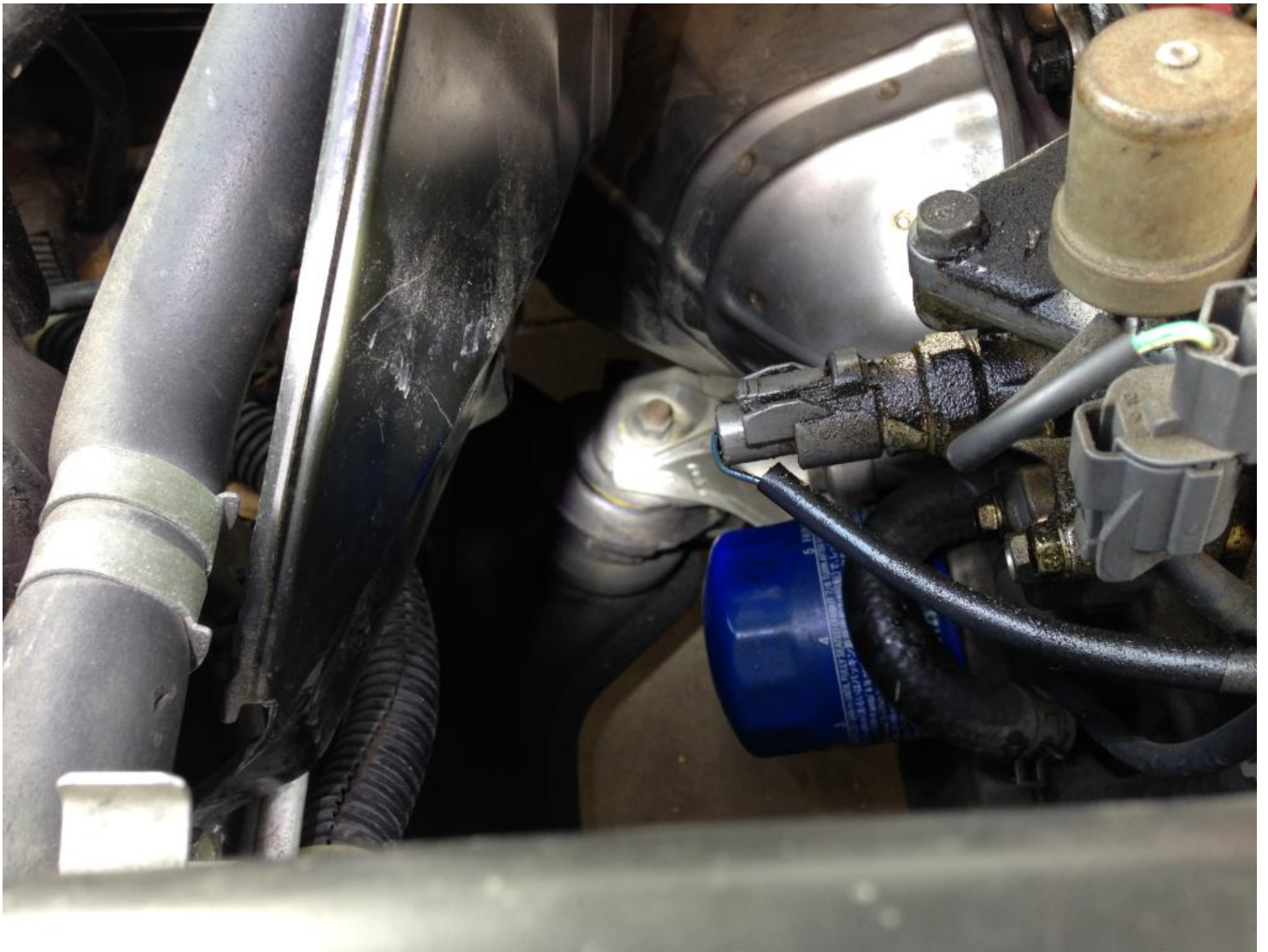
Removing the top nut (14mm)
